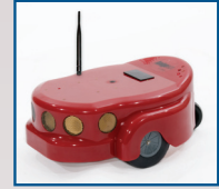
AmigoBot with Wireless Serial Ethernet for remote operations
