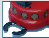
Amigo Fingers (Spring-loaded passive Grippers)
